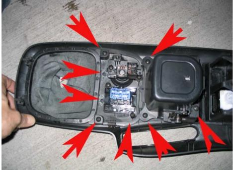
7)Next, take the roof button and reattach it. It pops right into the right sided hole (right side of the console when it turned over) and is held with two scres... just like the old one. Unfortunately, the old hazzard button doesn't fit...the button is too big and the housing is not correct for the new console. It appears honda used the same size for both the hazzard and roof buttons.
