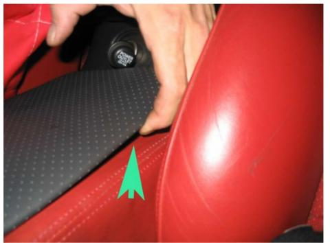
4) Unscrew the shiftknob and take it off. Once the console is up, disconnect the roof and hazzard light switches. There is a tab on each
