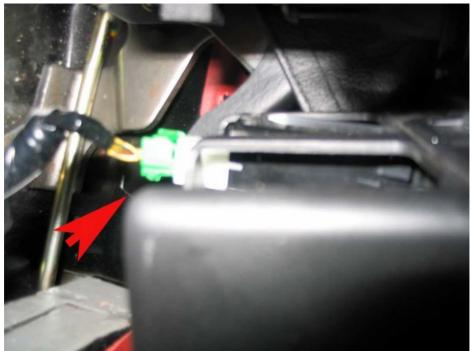
5)After those are disconnect. slide the console up and over the e-brake. You may have to move the e-brake into different positions, but the console comes right off.
